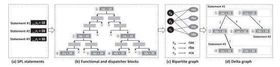
Fig. 3. Four major components of a BOP Compiler. The double and single border boxes ( $\square$ ) indicate functional and dispatcher blocks. The number inside a circle ( $\bigcirc$ ) represents the functional block number. The X represents irrelevant basic blocks.
